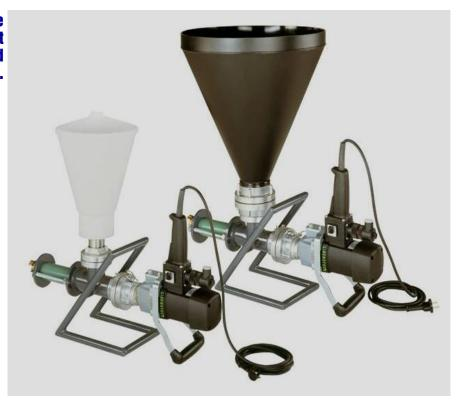
The unit can be equipped with upper containers of 6 or 30 litres volume. The delivery rate can be adjusted between 0,5 - 6 litres/minute by means of the electronically adjustable drive and can thus be easily adapted to the requirements on site.
