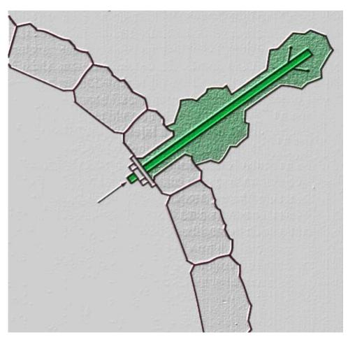
HydroBloc®PU 640 - The perfect anchor resin: thixotropic, fast setting reaction, high consistency. Bore anchor for injection, conventional anchor technique with steel or glass fibre reinforced anchors. Also for all applications where low viscous resins with fast setting time and high consistency is needed.
