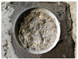
Concrete break at 5.4 N/mm<sup>2</sup> - adhesive tensile strength lab test without primer
