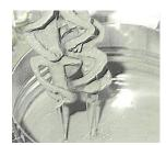
Empty component A completely into the container of component B and stir with a mixing machine until the colour of the mixture is even and free of streaks. Then repot the mixture as usual and mix thoroughly once again. Do not stir in air!
