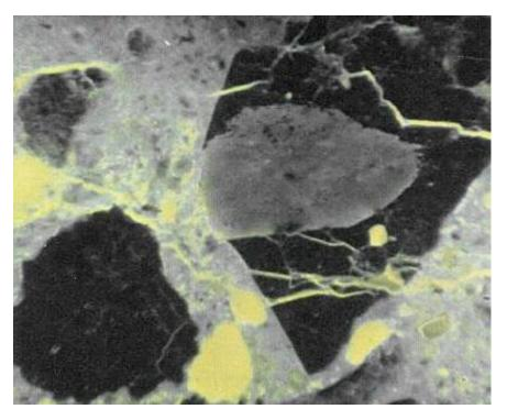
Silox®Injection 811nt: **Creeps into** micro cracks, finest pores and capillary structures
