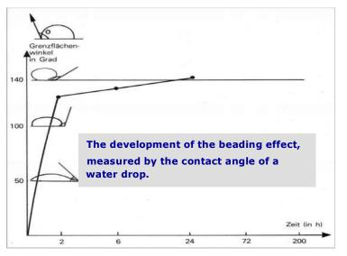
With 200 gr/m<sup>2</sup> material HydroBloc<sup>®</sup>Si-742-K aqua impregnated floor plate. Calibrated water drops were placed in regular distance on top of the treated floor. The developed contact angle was measured
