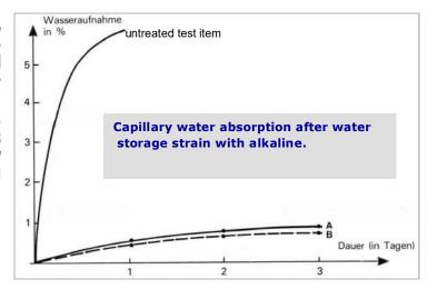
Test item made of cement mortar, impregnated with 400 gr/m<sup>2</sup> HydroBloc<sup>®</sup>Si-742-K aqua was stored under water and the water absorption was measured (ð Curve Å)
