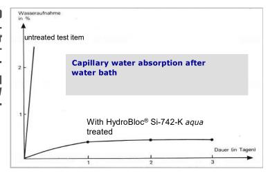
A brick impregnated with 400 gr/m<sup>2</sup> HydroBloc®Si-742-K aquastored in water 1 cm deep, water absorption through capillary sucking measured after 3 days.
