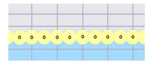
Principle of a typical horizontal barrier, with holes in a row and idealized barrier layer from the filling material
