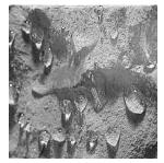
Due to this internal hydrophobization with silicone, the mineral building material is no longer wettable with water. The capillary water transport in the pores of the building material is interrupted.
