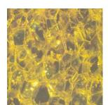
HydroBloc®510 is a classic 1 component injection foam with high reactivity. Activate the 1 component resin with an accelerator (HydroCat®513 or 514). After activation, the product reacts very fast with water, this happens with strong foaming, to an elastic and inherently stable PU foam. As far as possible, the PU foam has closed cells and does not shrink during the hardening process.
