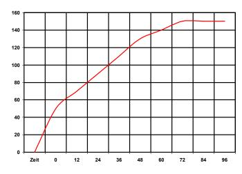
**Increase of volume** of HydroBloc®PU 500 reference block stored in water
