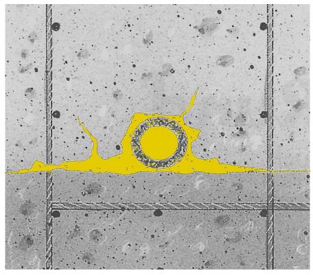
Honey-combs and cracks will be filled with injection resin completely. This will produce a watertight concrete structure.
