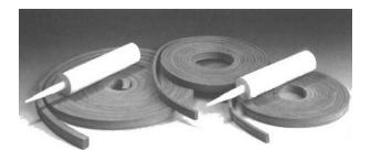
For installation on uneven or rough surfaces, use BentoMastic<sup>®</sup>307, the swelling tape from the cartridge. This avoids lateral infiltrations and leaks. On smooth, even surfaces, installation is carried out with BentoColl<sup>®</sup>305, an adhesive specially adapted to bentonite tapes. Alternatively, BentoFlex<sup>®</sup>Quellfugenband can also be nailed on.
