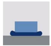
Quickly installed and doubly safe: BentoFlex®Quellfugenband glued with BentoMastic®307
