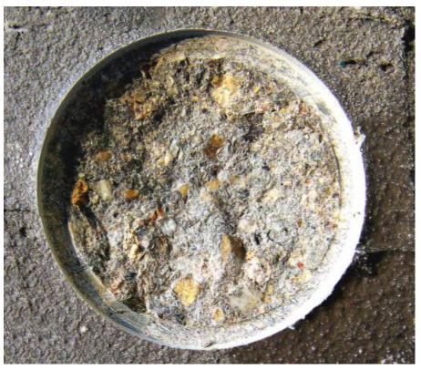
Silipox®Baukleber Burst in Concrete at 4,95 kN
