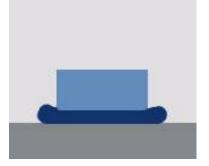
Quick installation with double safety: HydroTape®Quellfugenband glued with HydroSeal®355
