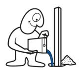
Anchor resins are injection resins made for anchoring bolts in rock or concrete. The fast setting and immediate high strength are ideal for the application.
