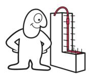
Injection hoses are the perfect solution for sealing joints, working joints, double walls and pipe penetrations. The injection resin seals the joint and the pore structure, honeycombs and cracks without additional drilling. Multiple injection is also possible after years. The best of the best is the Swellinjekt, the combination of high-quality polymer swelling tape and injection hose.
