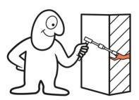
Foaming resins such as waterstop resins are very popular and regularly bring good success in stopping running water. Particularly 1-component waterstop foam is used a lot and often the necessary post-injection is dispensed with.
